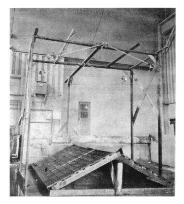
Figure 1. Rain test apparatus suitable for Method A (from ASTM D 2898-94).
